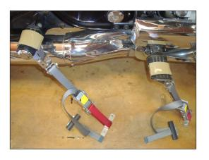
tie-down optimized for tie-down of the mid or rear section of M/C to cargo vehicle floor with a minimum of 9.0 inches of clearance. The opposite end of this tie-down has a peg-saddle loop F3X-PS to capture pegs. The F3X Mid-Frame tie-down has a operating length that allows the rider to secure the motorcycle into position from the seat before dismounting from bike.
